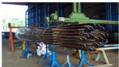
Tube Bundle - Oil Preheater
